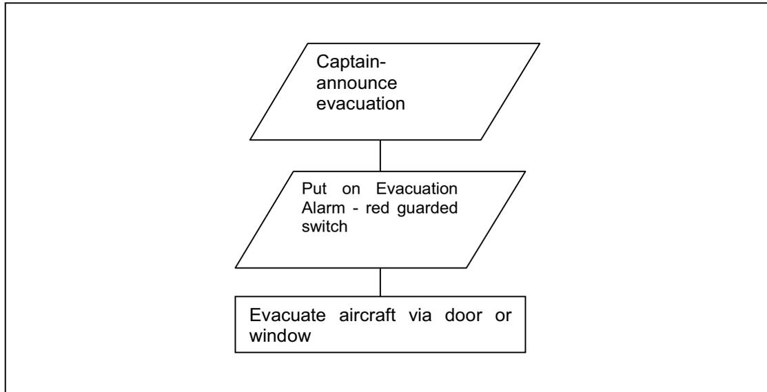
**Figure 18** Part of the emergency evacuation flow diagram
