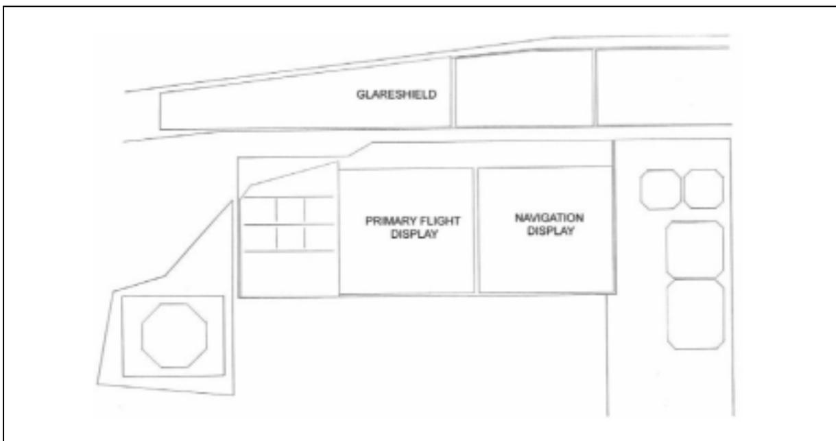
**Figure 25** Diagram of forward view of flight deck, left seat showing the main functions of the different instrument groups
