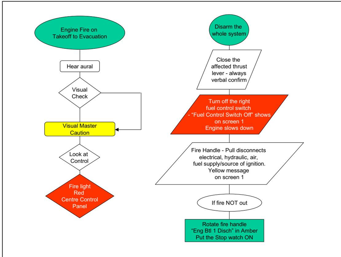
**Figure 19** Some of the controls and displays that appear in the full flow diagrams of the emergency procedures
