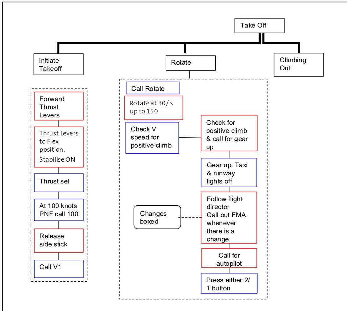
**Figure 9** Part of the task analysis showing where the pilot uses landing gear indicators (boxes marked red).
