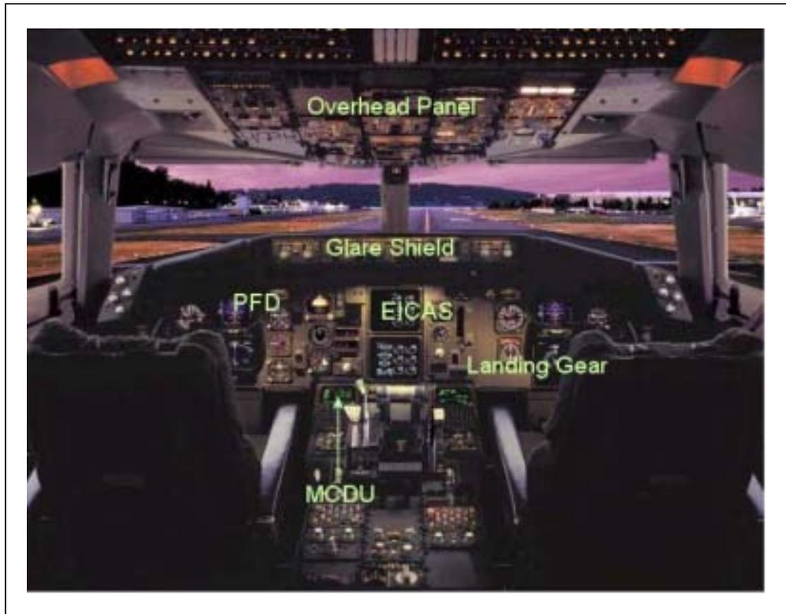
**Figure 16** Photograph of the main controls in the Boeing 757 flight deck
