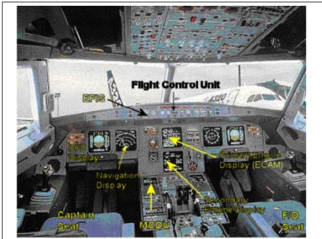
**Figure 3** View of the Airbus flight deck showing some of the key instruments discussed in the report. See main text for a more detailed description.
