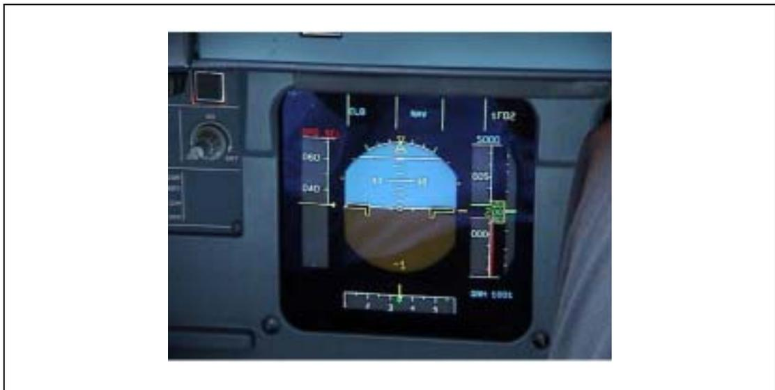
**Figure 14** Photograph of the Primary Flight Display
