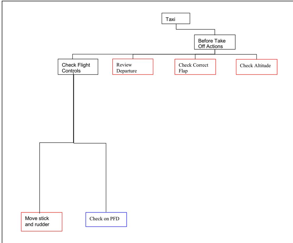
**Figure 12** Part of the task analysis to indicate where the pilot uses the flight director bars (See Figures 13 and 24 for layout of the primary flight display).
