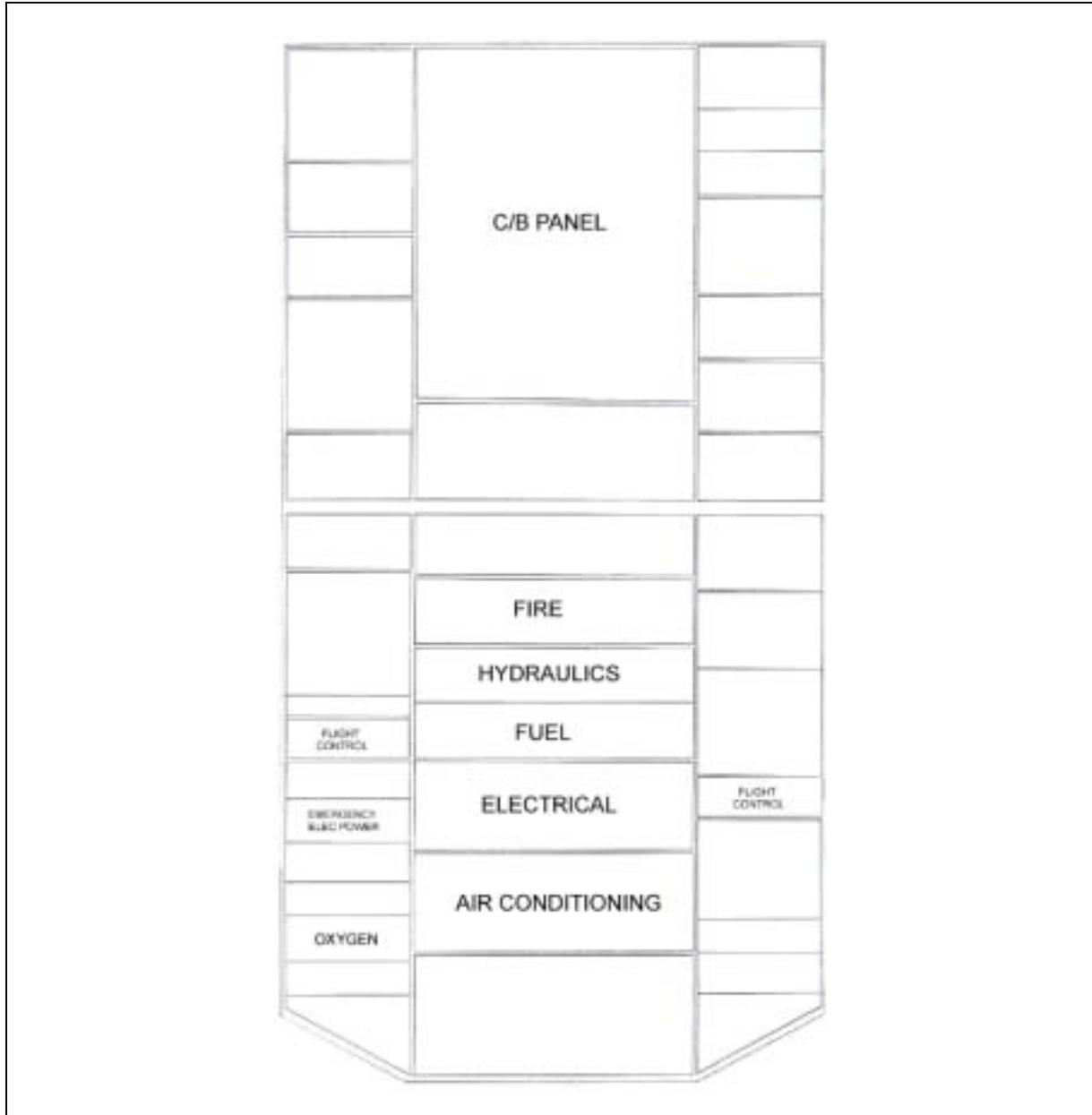
**Figure 23** Diagram of the flight deck overhead panel showing the main functions of the different areas
