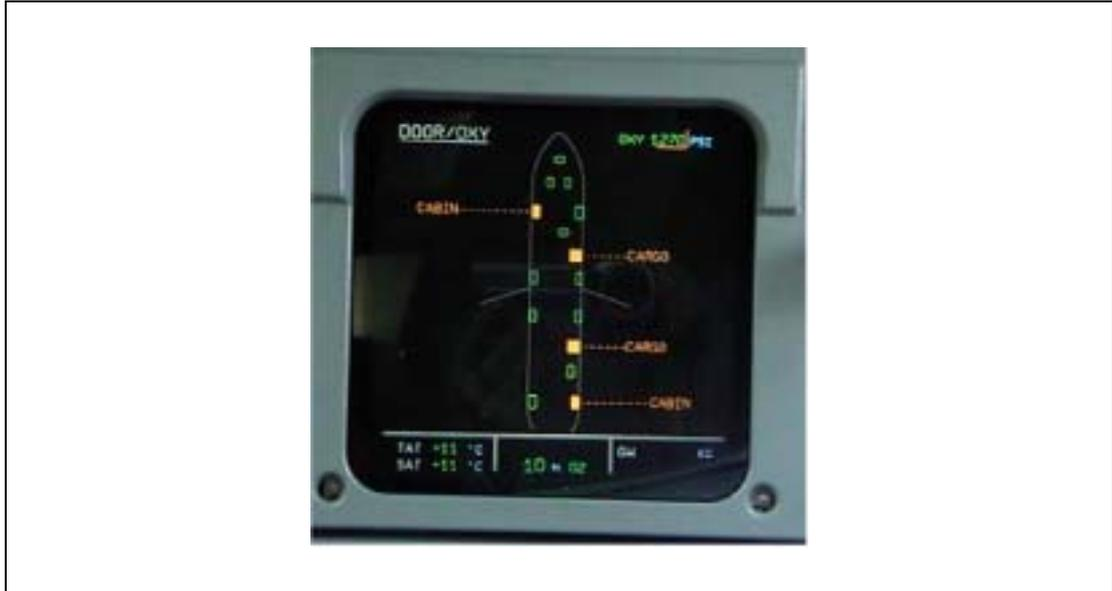
**Figure 11** Photograph of the ECAM door and oxygen page
