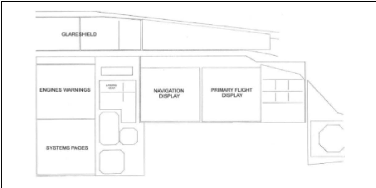
**Figure 24** Diagram of forward view of flight deck, right seat showing the main functions of the different instrument groups
