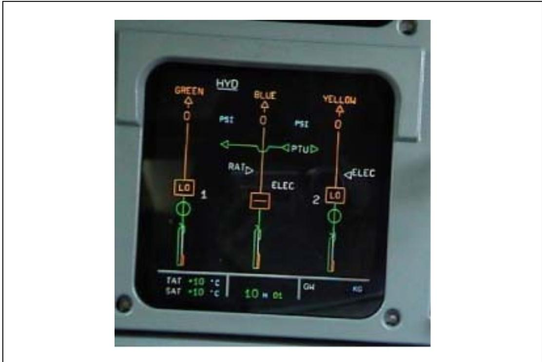
**Figure 8** Photograph of the ECAM hydraulic page.
