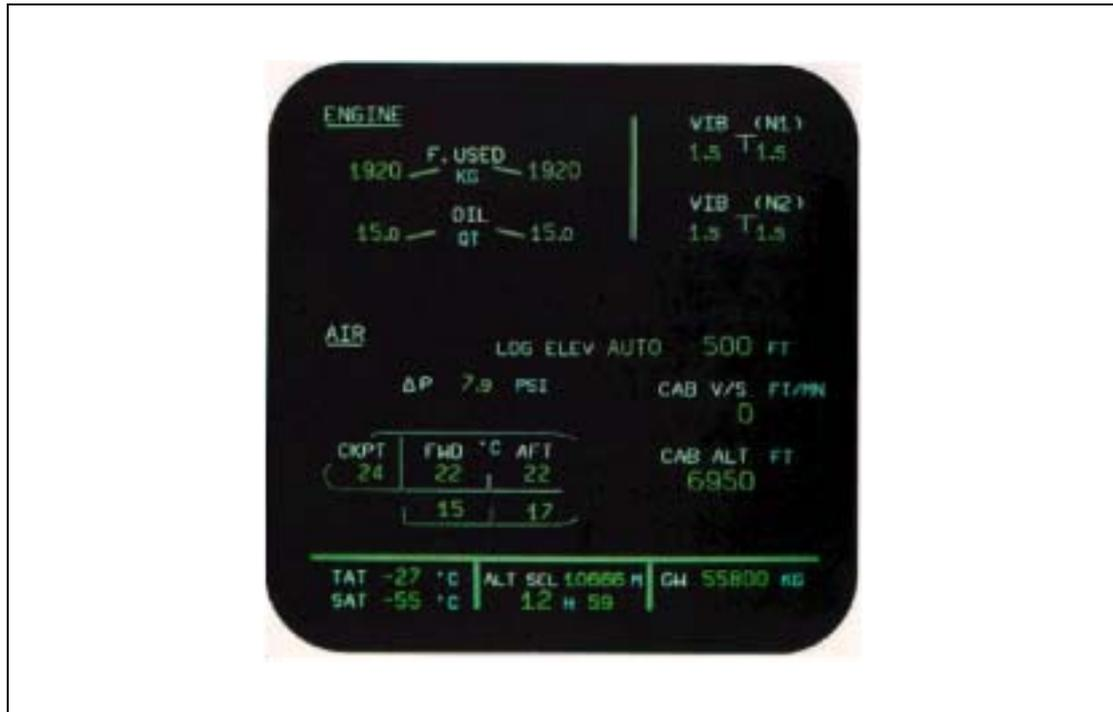
**Figure 4** An example page from the ECAM system
