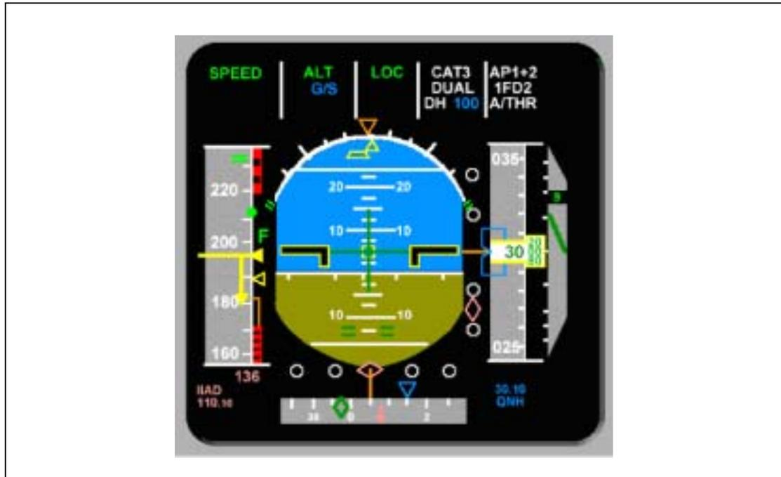
**Figure 13** Diagram of the Primary Flight Display. Red and black symbology provides information on low and high speeds.
