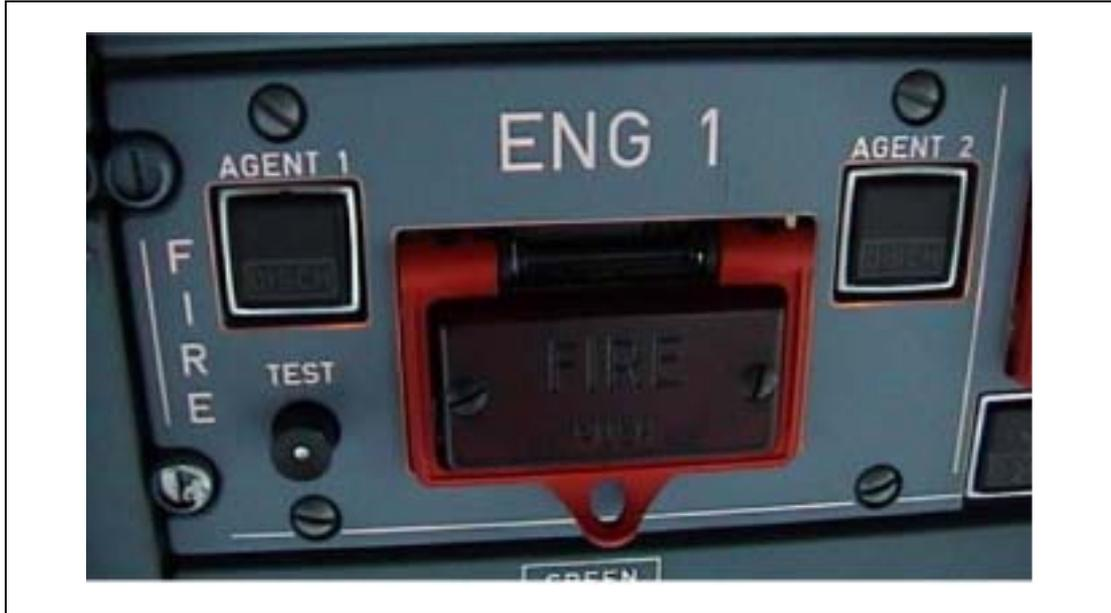
**Figure 5** Photograph of the engine 1 fire indicator and agent 1 and 2 lights. This panel is in the overhead panel.
