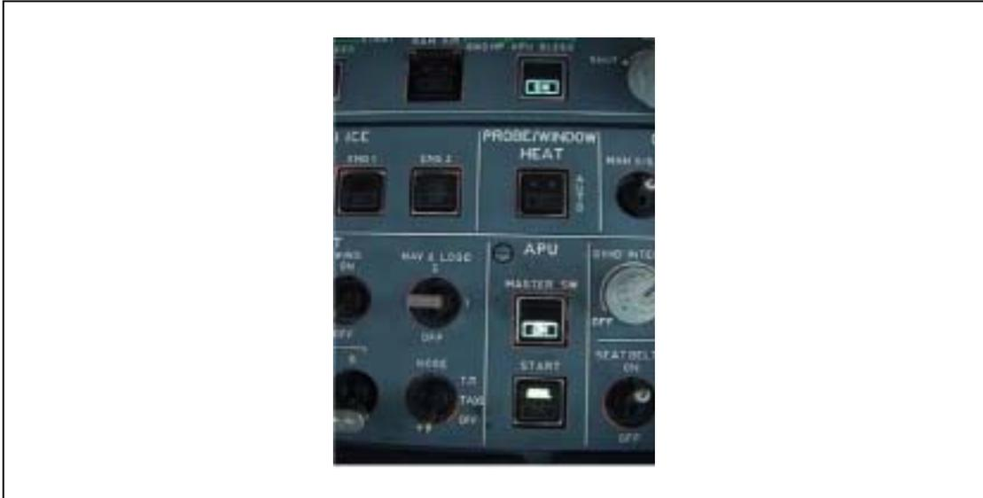
**Figure 10** APU Pushbutton (overhead panel), showing the blue backlit text.
