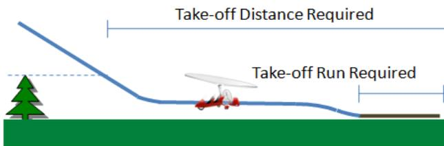
b) The gyroplane will run along the ground to achieve flying rotor speed, lift clear of the ground, and then accelerate (transition) a few feet above the ground to achieve the climb speed, and then enter the climb.
