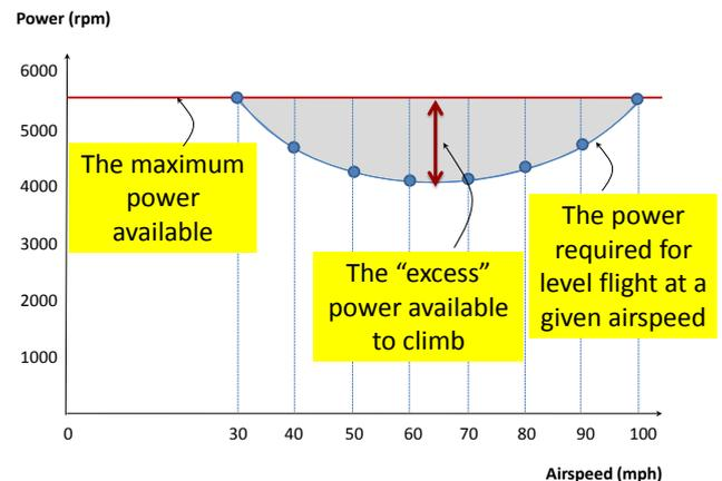
The values in the above diagram are for illustration only – refer to the flight manual for your gyroplane
