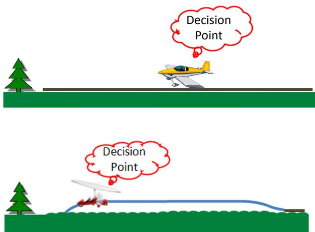
Pilots need to understand their aircraft, including the stopping distance. It is unlikely to be too late to abort a take-off in a gyroplane; most can stop in a matter of metres if flown properly.
