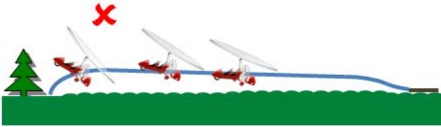
e) If the gyroplane is approaching an object within the clearway whilst still accelerating to best climb speed, it is an extremely natural human reaction to bring the stick backwards to aim the gyroplane over the obstacle. A pilot may try to force the gyroplane to climb over the obstacle. THIS WILL NOT WORK. Bringing the stick back without sufficient airspeed will simply increase the rotor drag and even with 100% engine power the gyroplane will descend, nose high, to the ground.
