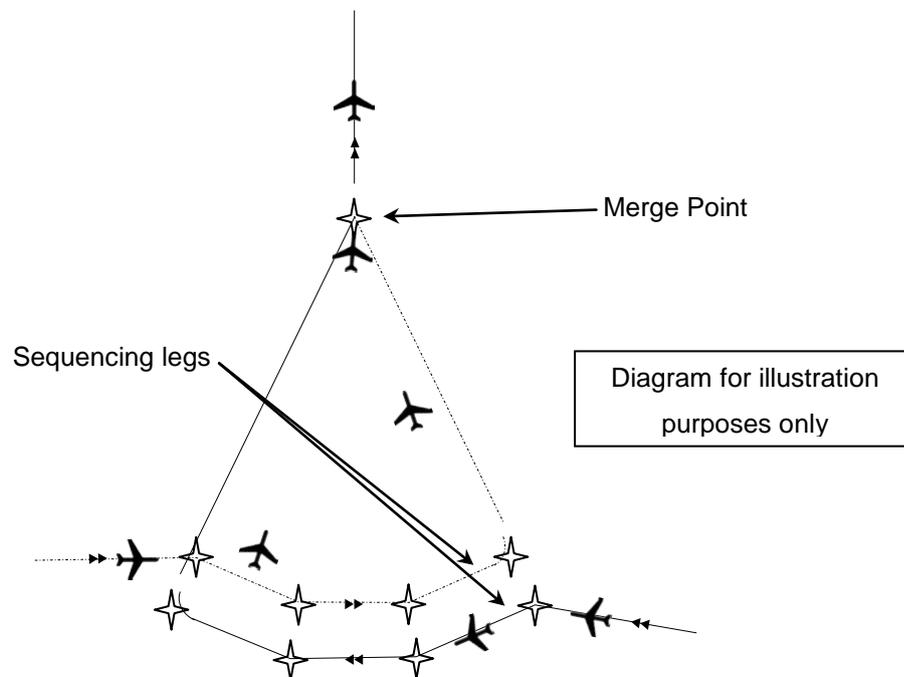
**Figure 1 - Point Merge Procedure**
