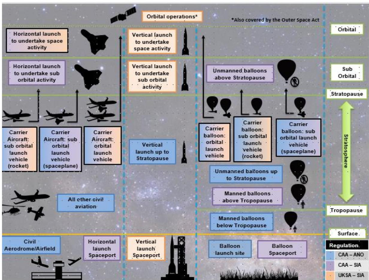
Rocket spacecraft are spacecraft that derive thrust from using a rocket engine and space planes are winged vehicles that act as an aircraft while in the atmosphere and a spacecraft while in space. Table 2 presents an overview of the types of spacecraft, operations, take off launch utilised and main power sources.
