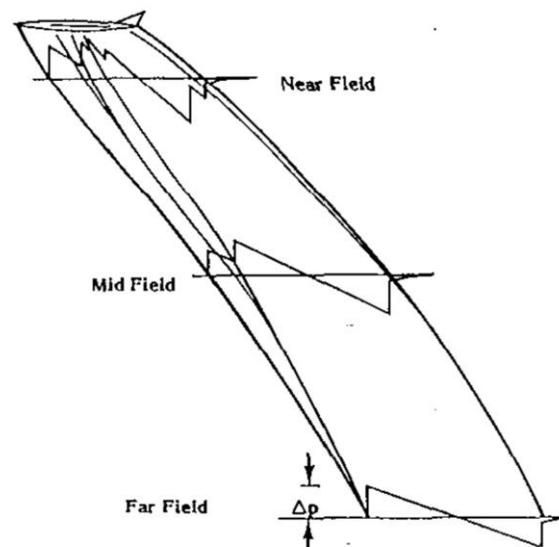
Design improvements to the shape of an aircraft cross-section can alter the N-wave signature to reduce the peak and soften the sound of the boom to an acceptable level. This will potentially enable supersonic flight over land. A level of acceptability of sonic booms has yet to be determined and may only be established by flying a demonstrator aircraft having a low-amplitude shaped signature over communities<sup>31</sup>.
