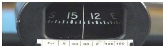
d) Check your DI for precession against the magnetic compass (remember the inherent errors), try to ensure level, balanced flight when synchronising and double-check using line features parallel to track.
