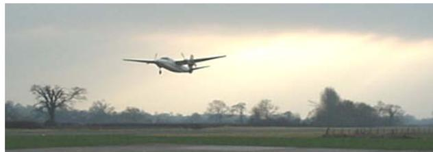
Under limiting conditions an engine failure shortly after lift-off may preclude continued flight and a forced landing will be necessary. Where the performance is marginal, consider the following points when deciding the best course of action:
