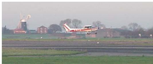
b) Landing on a wet surface, or snow, can result in increased ground roll, despite increased rolling resistance. Tyre friction reduces, as does the amount of braking possible. Very short wet grass with a firm subsoil will be slippery and can give a 60% distance increase (1.6 factor).
